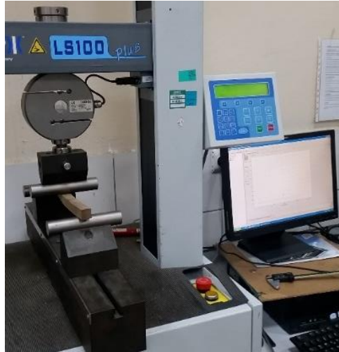
Figure 2. Performing bending test
