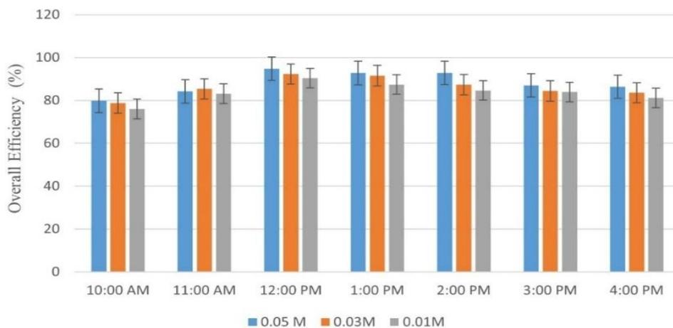
Figure 10. Variation of the overall efficiency measured on an hourly basis from the photovoltaic thermal system.
