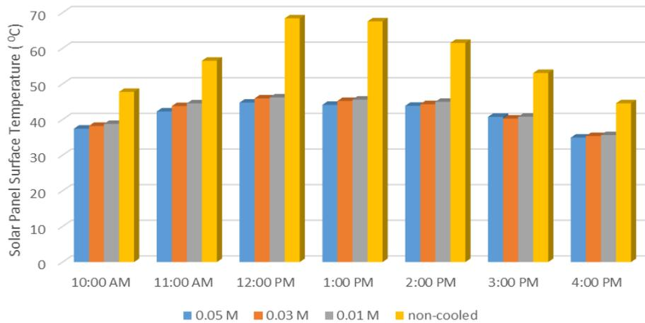
Figure 4. Changes in the surface temperature of photovoltaic panels on an hourly basis using nanofluid cooling and non-cooled system (photovoltaic system).
