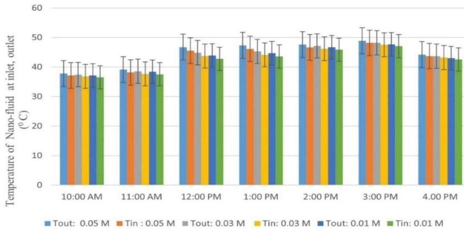
Figure 8. Fluctuations in the nanofluid inlet and outlet temperatures on an hourly basis.
