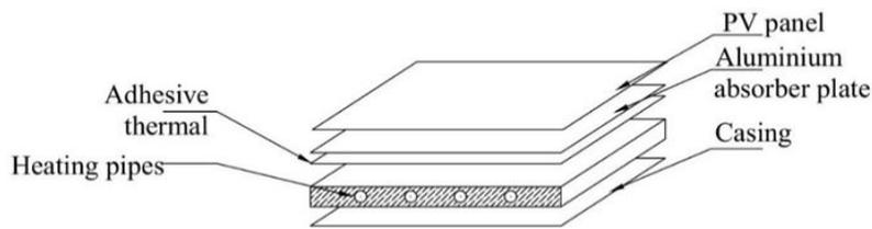
Figure 1. Cross-sectional view of the components of photovoltaic-thermal hybrid system.
