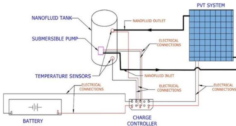
Figure 2. Component diagram of photovoltaic thermal hybrid experimental system.
