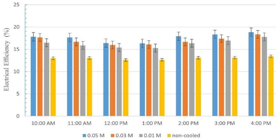
Figure 7. Fluctuations in electrical efficiency with time.
