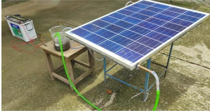
Figure 3. Photograph of the photovoltaic thermal system in working condition.
