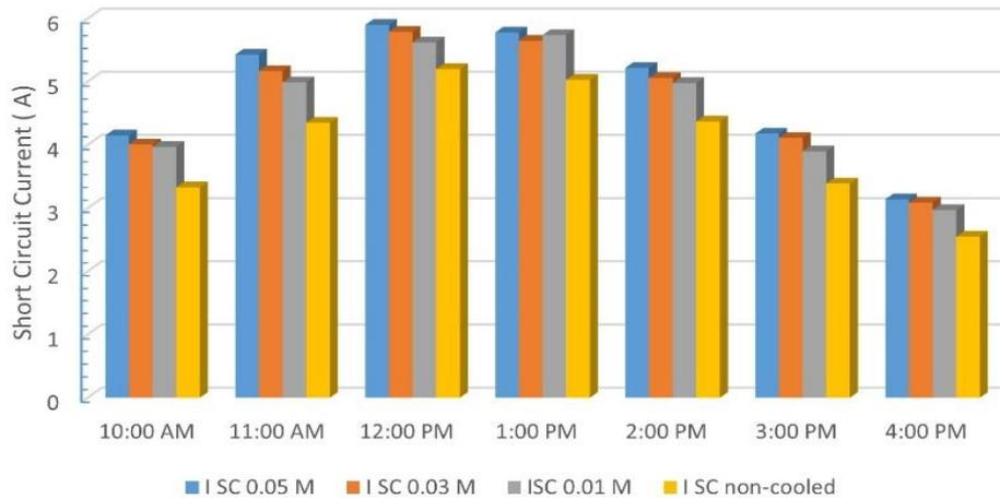
Figure 5. Fluctuations in photovoltaic thermal hybrid panel short circuit current over time in a cooled and non-cooled system.
