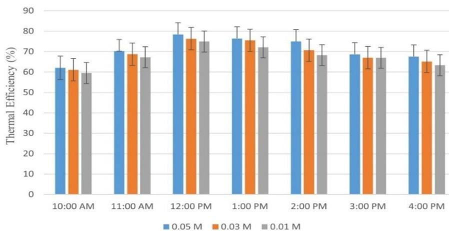
Figure 9. Fluctuations in the photovoltaic thermal hybrid panel thermal efficiency on an hourly basis.
