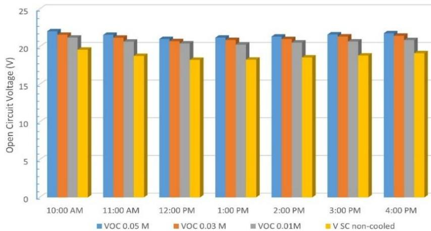
Figure 6. Fluctuations in photovoltaic thermal hybrid panel-open circuit voltage over time in a cooled and non-cooled system.
