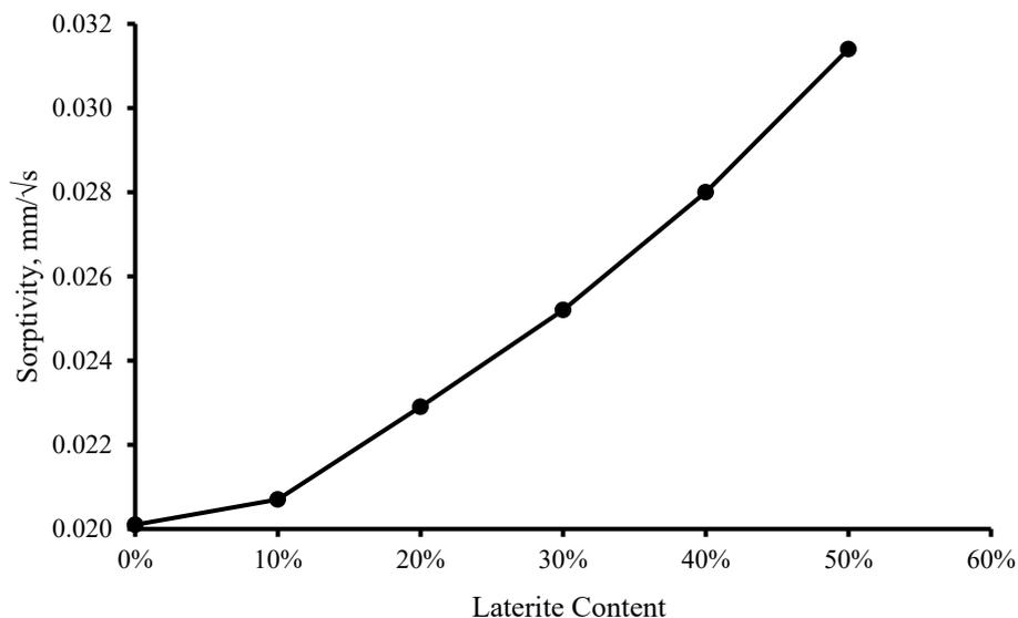
**Figure 5.** 28-Day Sorptivity of concrete with different laterite content under water immersion conditions
