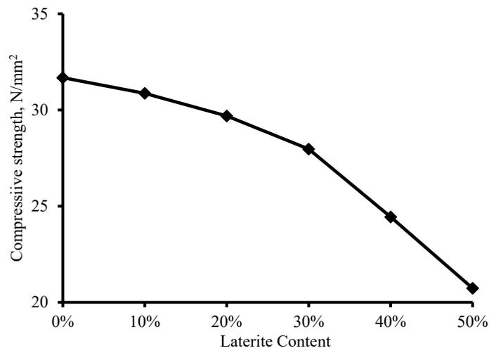
**Figure 3.** 28-day Compressive strength variation of concrete with varying laterite content in water immersion condition
