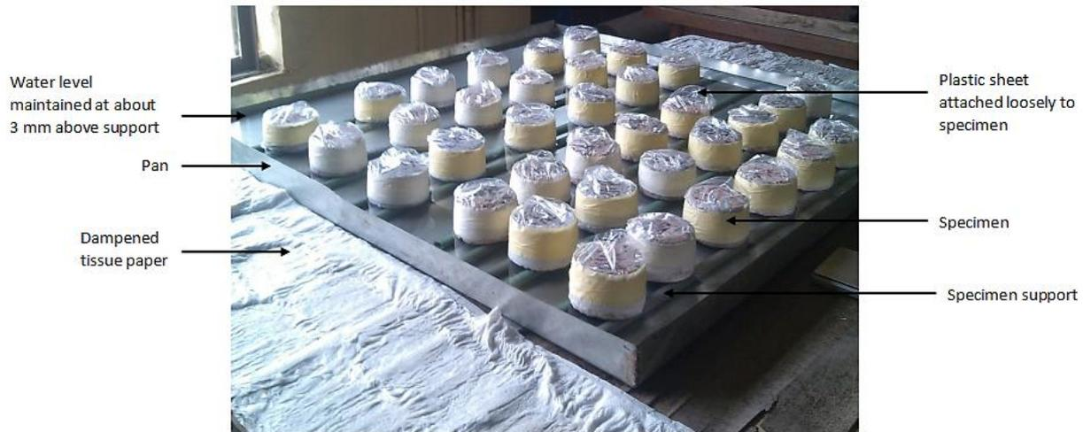
**Figure 2.** The sorptivity test system
