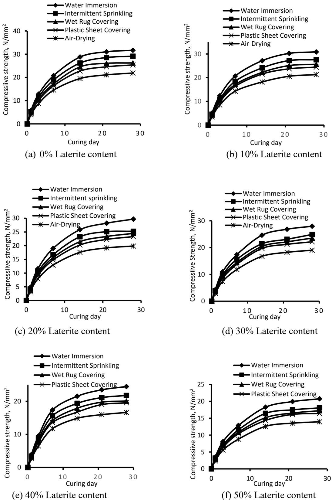
**Figure 4.** Compressive strength variation of concrete (encompassing varying laterite replacement levels) with different curing conditions and ages
