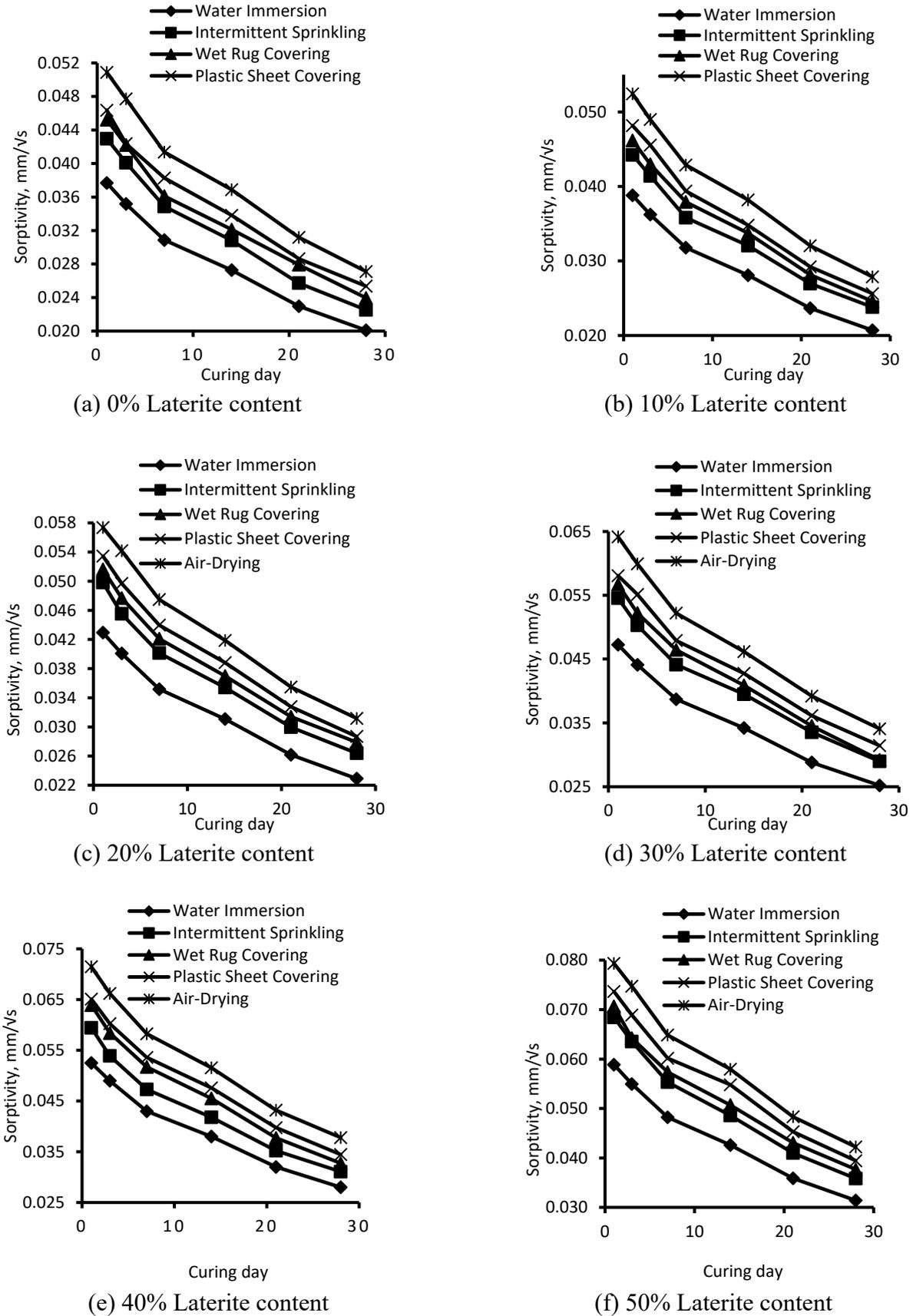
**Figure 6.** Sorptivity variation of concrete (incorporating varying laterite replacement levels) across different curing conditions and ages
