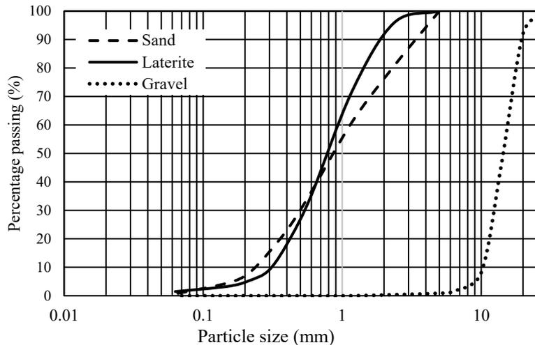
**Figure 1.** Gradation curves of the aggregates
