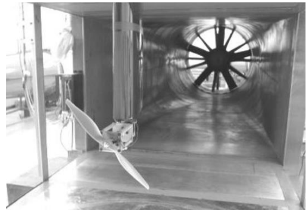
Figure 4. Wind Tunnel Used for Propeller Testing [6]
