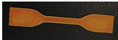
Figure 3. 3D printed tensile test sample
