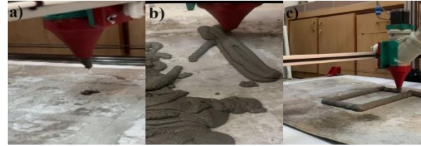
Figure 2. a) Flow Table Diameter Value Below 15 cm b) Flow Table Diameter Value Above 19 cm c) Flow Table Diameter Value Between 15-19 cm
