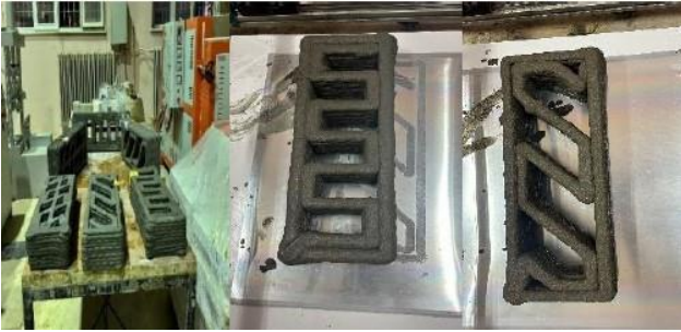
Figure 5. 3D Printed Hollow Concrete Beams
