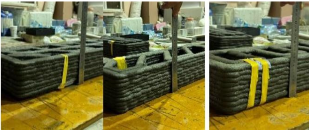
Figure 7. Hardened State Height Measurement
