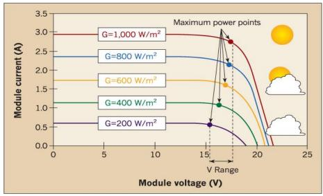
Fig. 7. A PV module's current versus voltage curve varies with the irradiance of sunlight [23].
