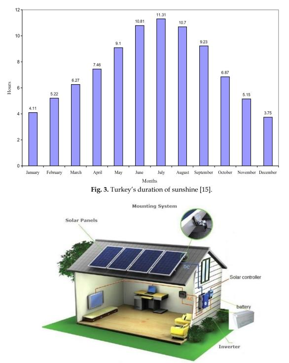
Fig. 4. Off-grid residential solar PV system [16].
