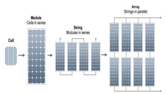
Fig. 6. From solar cell to solar array [19].
