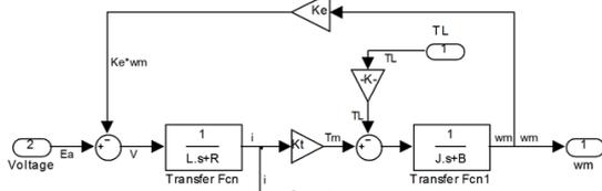
Figure 1. DC motor model in MATLAB Simulink.
