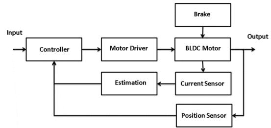
Figure 3. Block Diagram of System.
