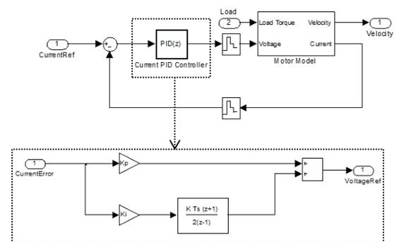
Figure 4. DC motor current control loop.
