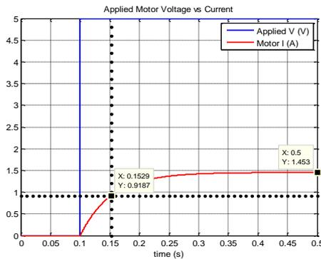
Figure 2. Applied motor voltage vs. current, with current value at 1 time constant ( $\tau$ ) marked.
