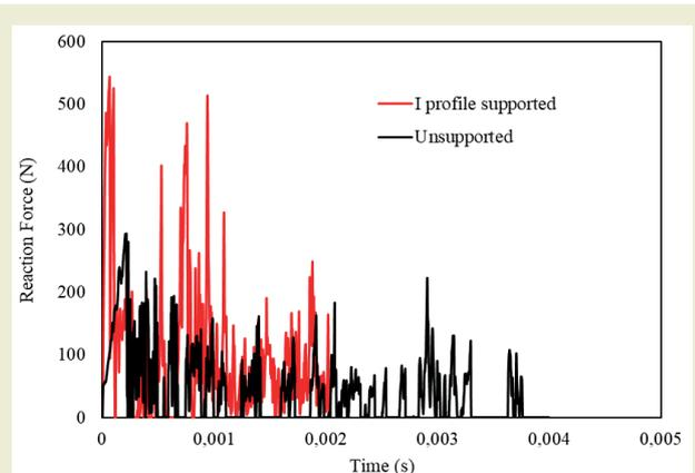
**Figure 6.** Reaction force-time graph of supported, and unsupported U-profile composites.
