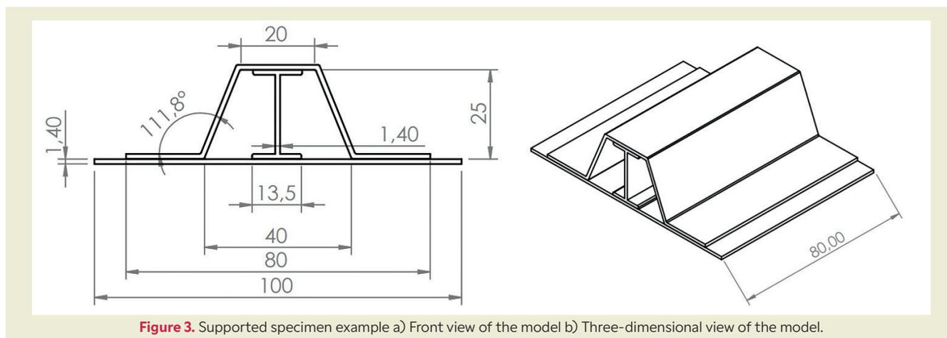
Figure 3. Supported specimen example a) Front view of the model b) Three-dimensional view of the model.
