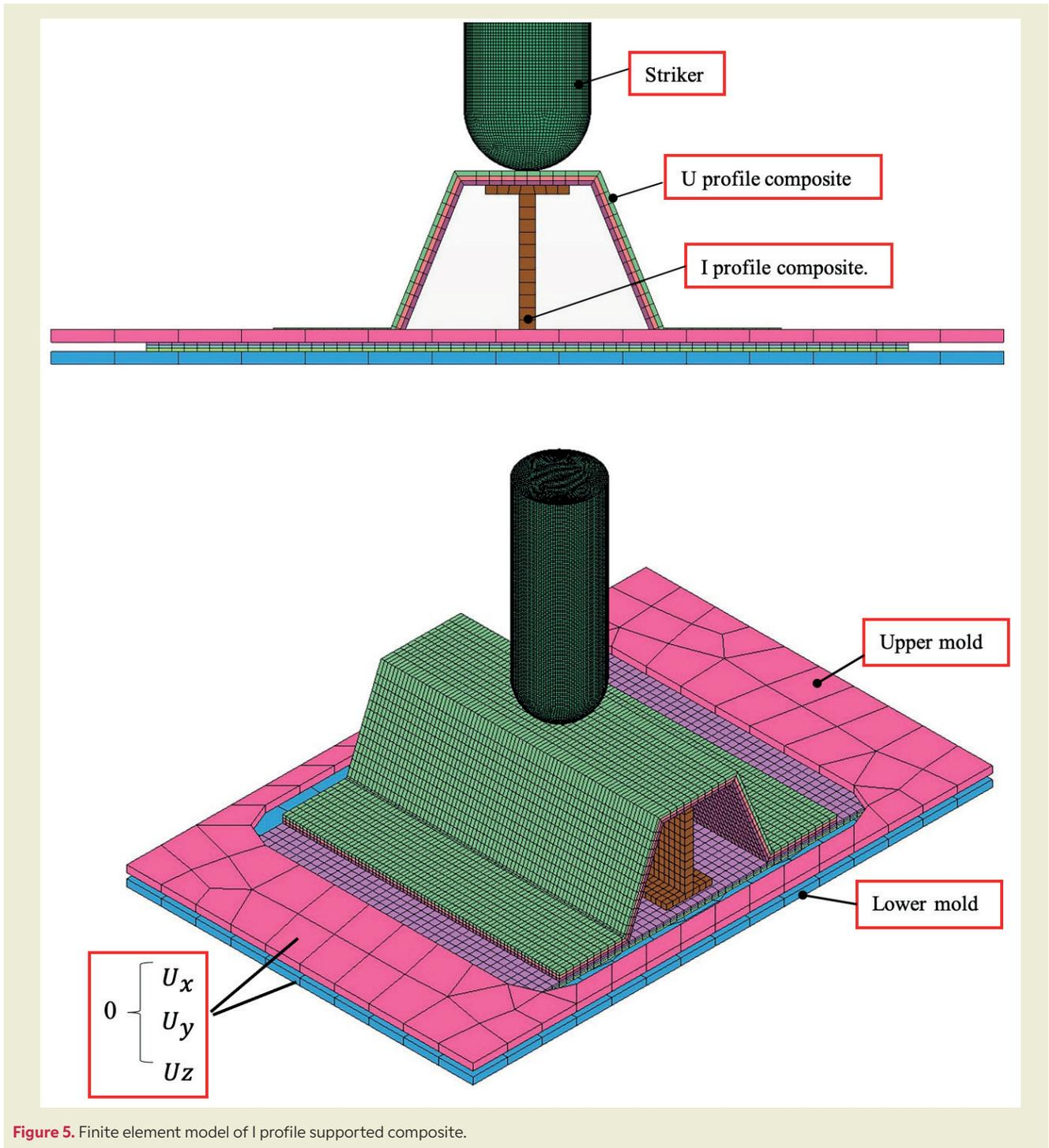
Figure 5. Finite element model of I profile supported composite.
