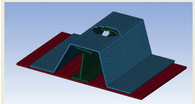
**Figure 9.** After-impact image of the I profile supported U-profile composite.
