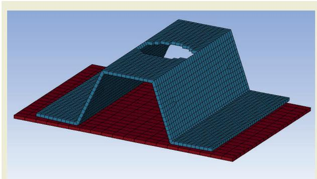
**Figure 8.** After-impact image of the unsupported U-profile composite.
