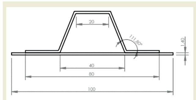
Figure 2. Front view of unsupported composite model.
