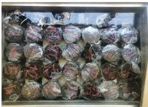
Figure 4. Wrapping and incubation of specimens with stretch film
