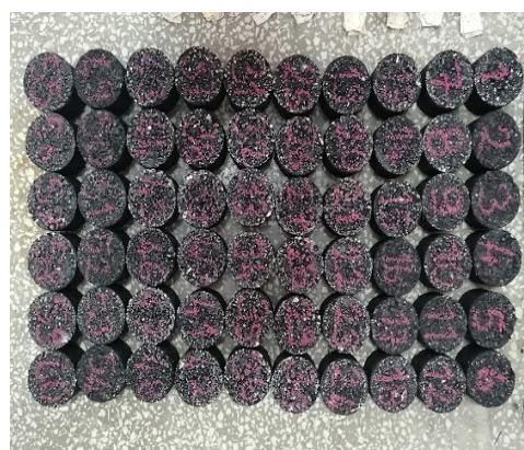
Figure 8. Appearance of some of the samples subjected to the moisture damage test
