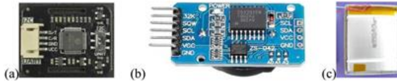
Figure 3 (a) Heart Rate and Oximeter Sensor board (b) DS3231 RTC module (c) Power supply
