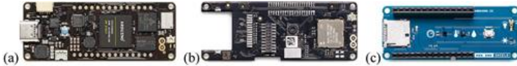
Figure 2 (a) Arduino Portenta H7 board (b) Arduino Portenta Vision Shield board (c) ENV Shield board
