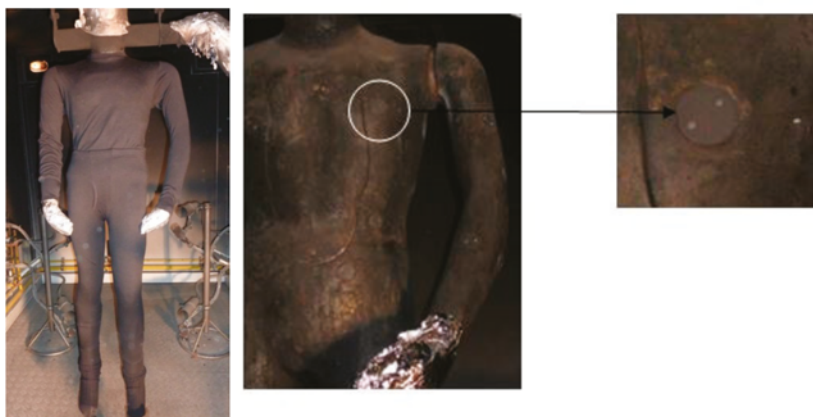
Fig. 6 Used thermal mannequin and temperature sensor [18]
