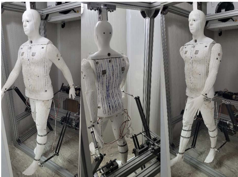
Fig. 10 Thermal Mannequin System Produced with 3D Printer [20]
