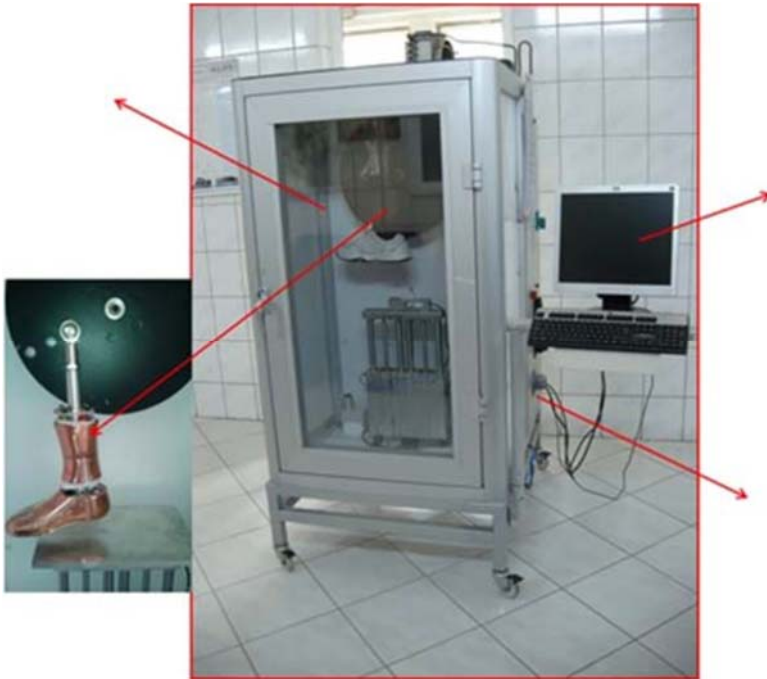
Fig. 18 Thermal foot mannequin system [30]
