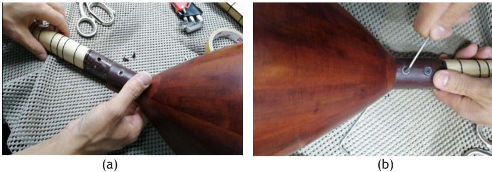
Figure 5. Connecting the neck to the soundboard (a) placing and (b) screwing the neck
