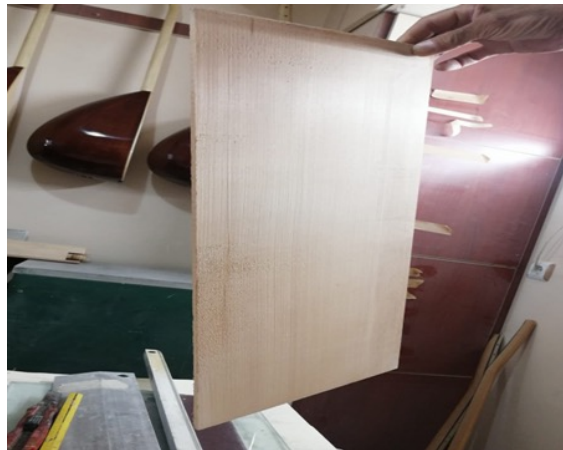
Figure 7. A piece of spruce tree for the soundboard
