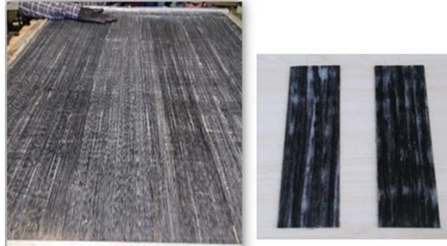
Figure 5: Laminated carbon fiber reinforced composite plate and [0^\circ/90^\circ/0^\circ] stacked sandwich face plates
