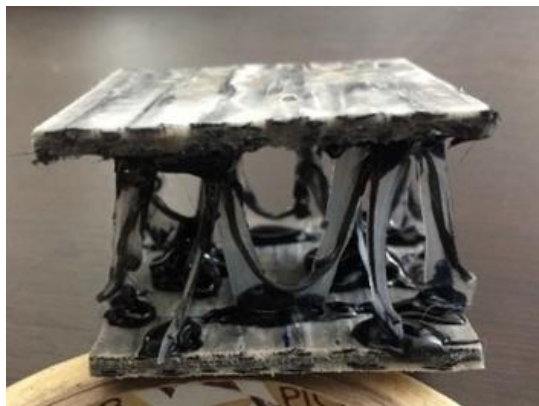
Figure 10: Sandwich specimen for flatwise compression test
