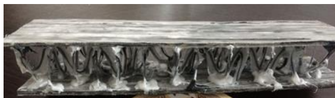
Figure 12: 3-point bending specimen of sandwich structure
