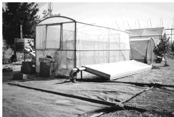
Figure 1. View of new designed solar tunnel dryer.
