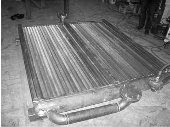
Figure 6. Pressure test of the heat exchanger
