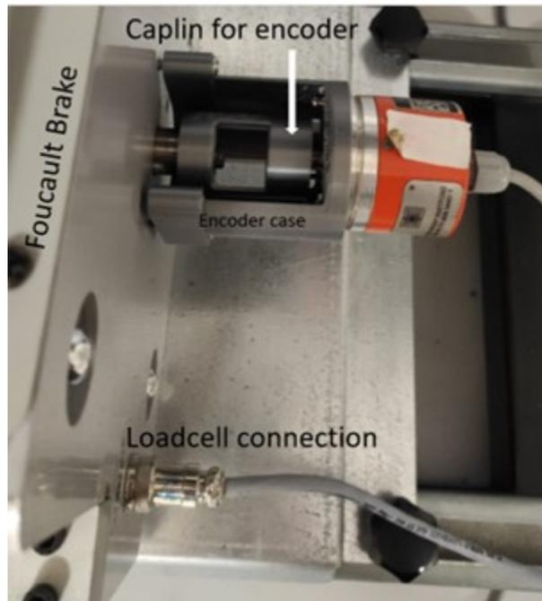
FIGURE 4. **Incremental encoder with foucault brake and connections.**
