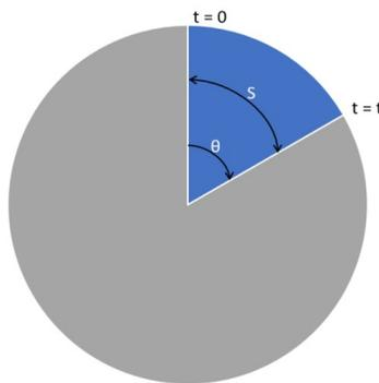
FIGURE 2. Angular displacement.
