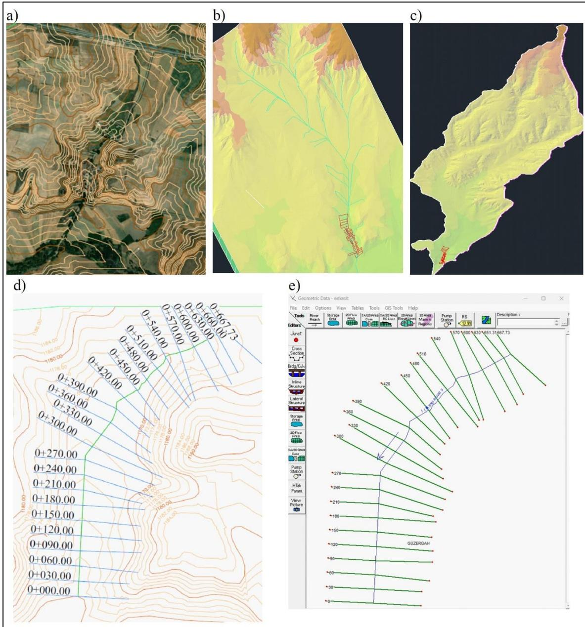
**Figure 5.** (a) 1/25000 Digital Elevation Map of the study area, (b) 3-D map, (c) basin area, (d) plan view of selected cross-sections in the study area (e) plan view in HEC-RAS
