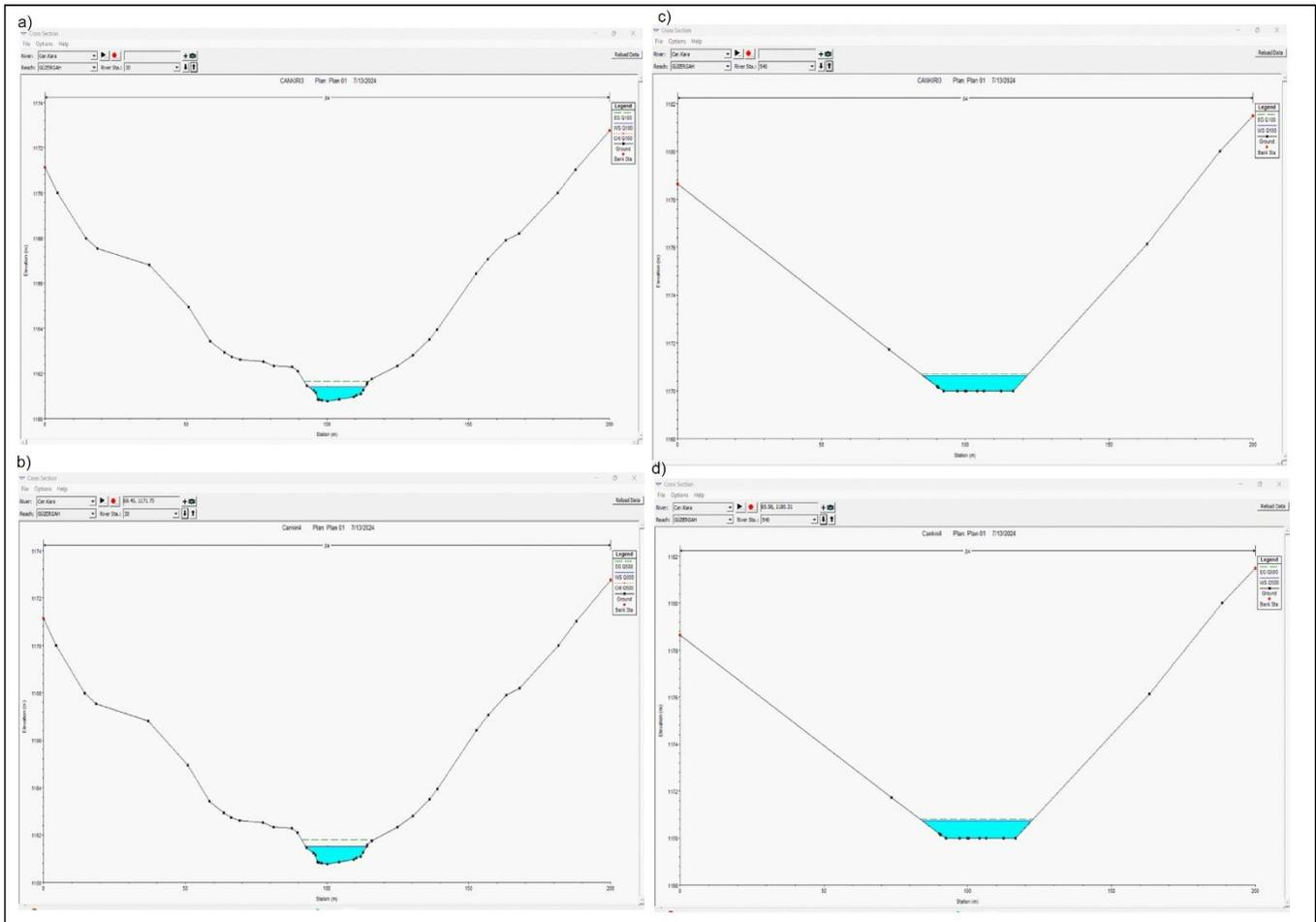
**Figure 6.** Channel cross-section examples (a)  $Q_{100}$  water surface profile at cross-section (30 m) with water level at 1161.40 m, (b)  $Q_{500}$  water surface profile at cross-section (30 m) with water level at 1161.59 m, (c)  $Q_{100}$  water surface profile at cross-section (540 m) with water level at 1170.65 m, (d)  $Q_{500}$  water surface profile at cross-section (540 m) with water level at 1170.78 m.
