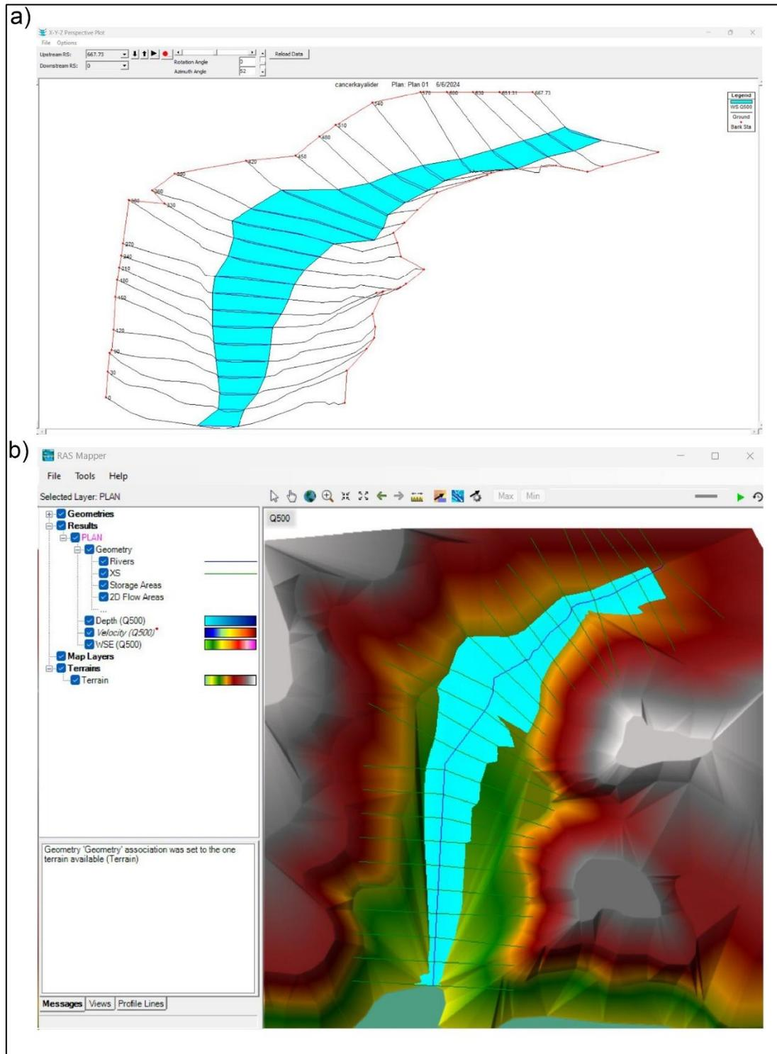
**Figure 7. (a)  $Q_{500}$  water surface profile created with HEC-RAS, plan view, (b) RAS mapper view**
