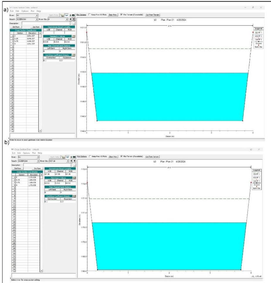
**Figure 10.** Cross-section view of the designed channel and flood level (a) upstream (b) downstream
