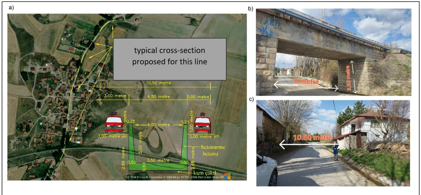
Figure 9. (a) Plan view of the designed channel, (b) railway culvert dimensions, (c) minimum road width
