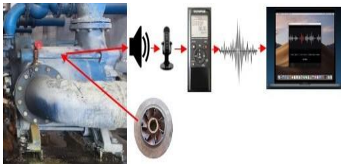
Fig. 3. Cross-sectional picture of the centrifugal pump under listening
