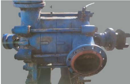
Fig. 1. Front view of three-stage horizontal shaft centrifugal pump
