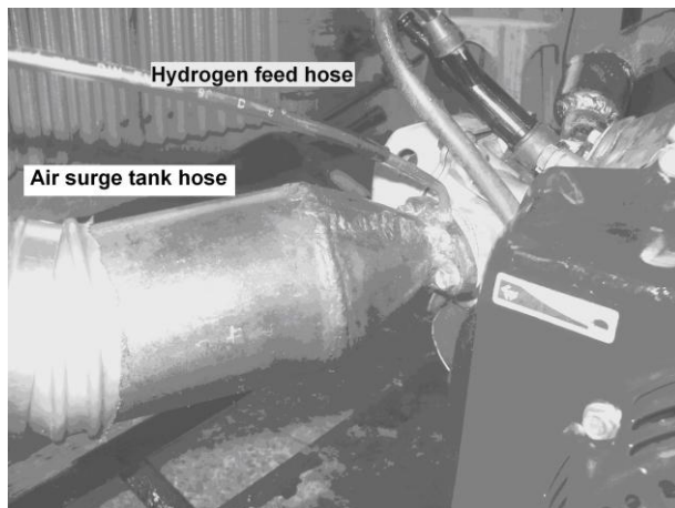
Figure 2. Induction of hydrogen to the engine.
