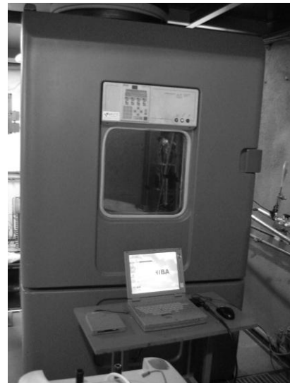
Figure 1. Climatic chamber used for simulation of ambient conditions.
