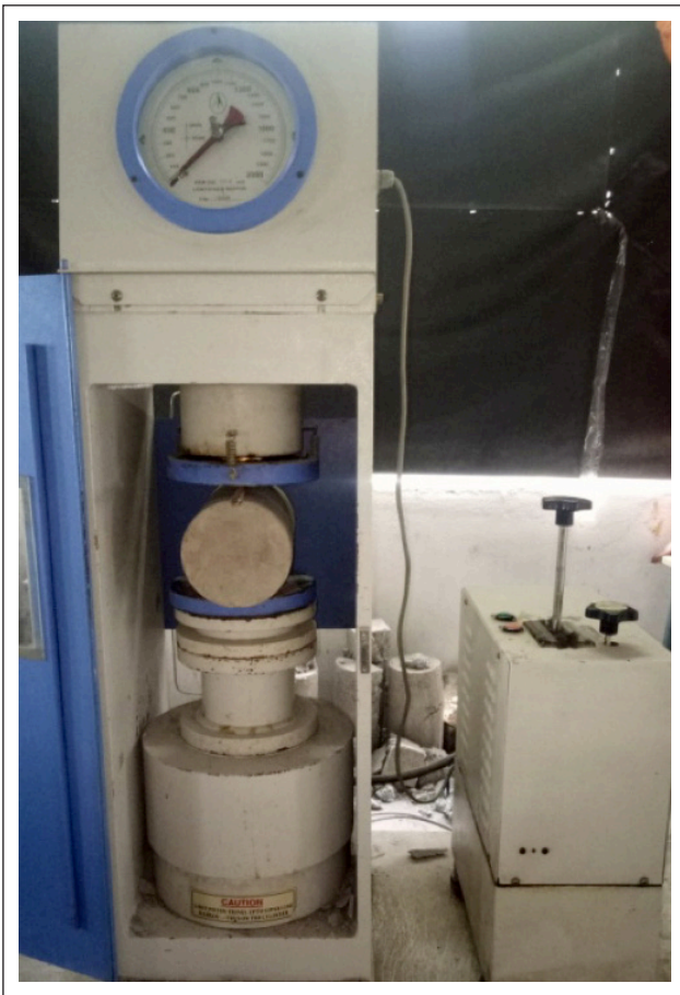
Figure 6. Experimental photograph of Split tensile strength test.
