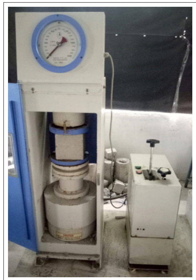
Figure 5. Experimental photograph of compressive strength test.
