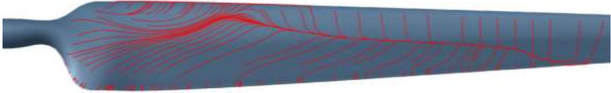
Figure 7. Skin-friction lines on the suction side of NREL Phase VI blade. ( V = 10 \text{ m/s} , k-\omega SST turbulence model)
