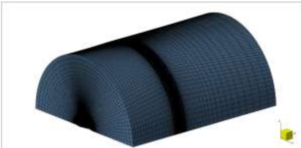
Figure 3. External view of the mesh with 3.41 million points
