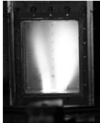
Figure 5. Visible flame luminosity for the test case, Re_{Dh}=19400 , Sw=0.74 , \phi=0.7 , (Tunçer et al., 2014)
