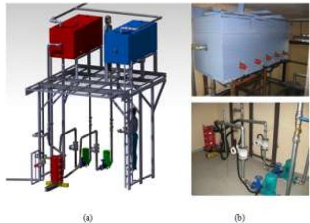
**Figure 1.** (a) 3-D CAD model of the test set-up, and (b) Views of the set-up (hot water tank, pumps, flow meters, heat exchanger and the connections).
