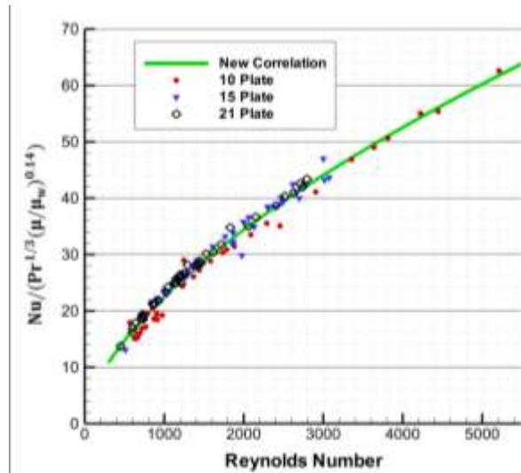
**Figure 6.** Nusselt number vs Reynolds number for different number of plates: new correlation and comparison with the experimental data.
