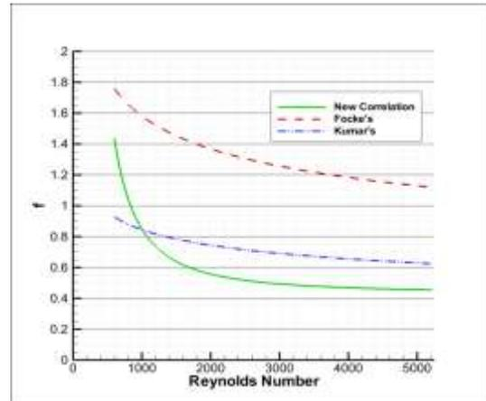
**Figure 9.** Comparison of new correlation curve for friction factor with existing correlations in literature.
