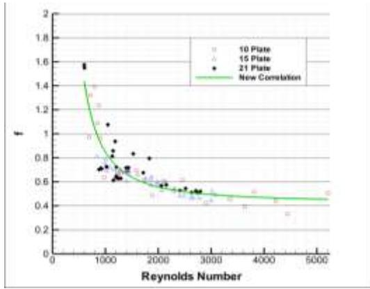
**Figure 8.** Friction factor coefficient vs Reynolds number: Experimental data for different number of plates and new correlation.
