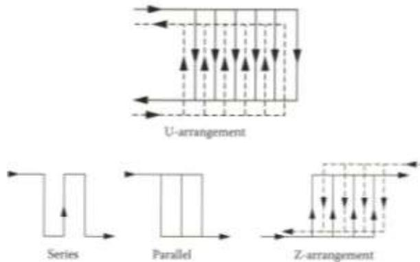
Figure 3. Flow pattern: (a) Schematic of a U-type arrangement – counter flow, single-pass flow (1x6/1x6) (b) Z-arrangement (1x4/1x4 configuration) [1]
