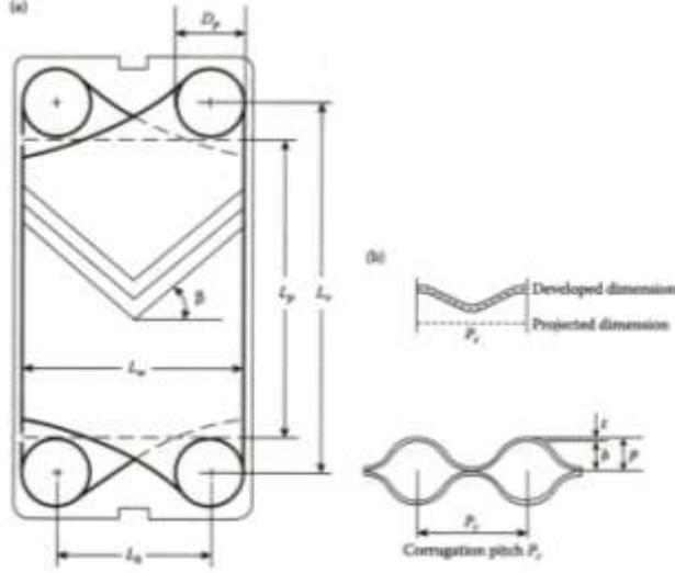
**Figure 4.** (a) Main dimensions of a chevron plate; (b) developed and projected dimensions of a chevron plate cross-section normal to the direction of troughs [1]
