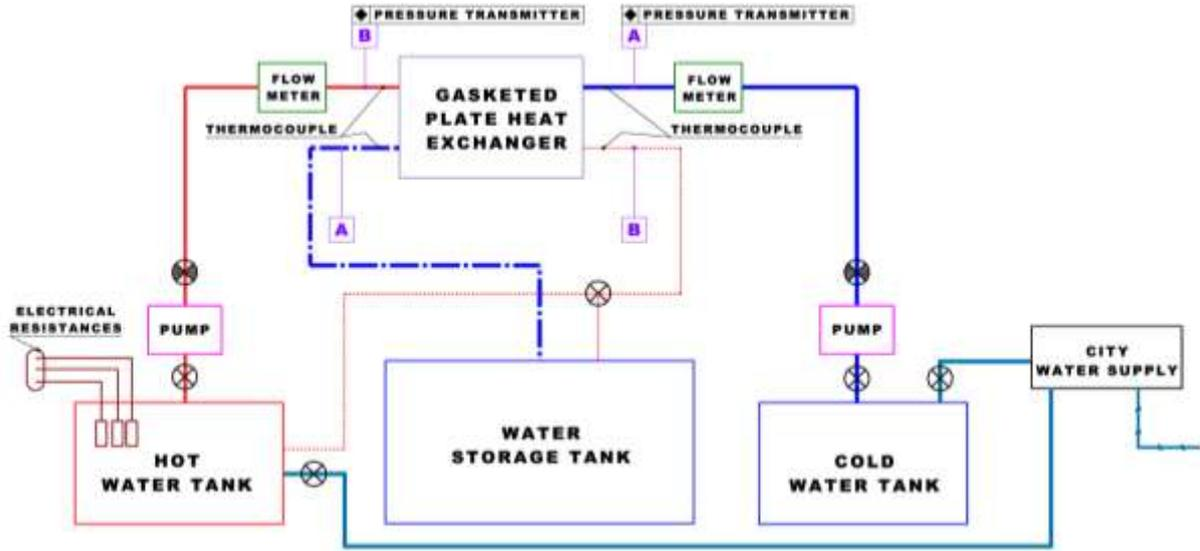
Figure 2. Schematic view of experimental test set-up.
