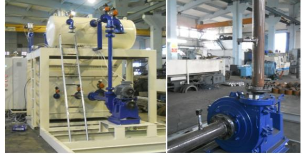
Figure 5. The experimental set-up (left) and the slurry pump (right), (Tufekcioglu Kaucuk Ltd., 2012)
