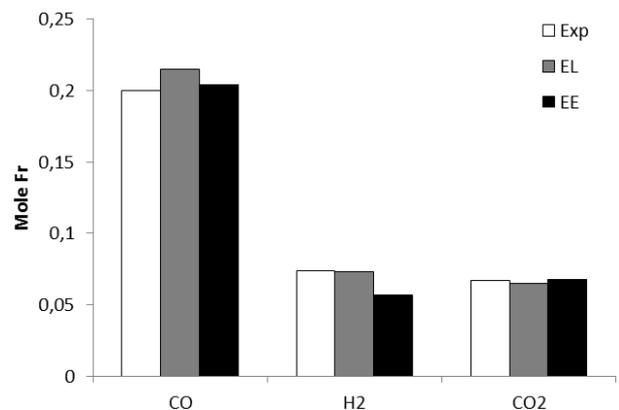
Figure 4. Mole fractions at gasifier outlet (AR=0.40, SR=0.0).
