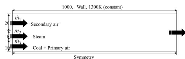
**Figure 1.** Schematic of tubular gasifier (dimensions in mm).
