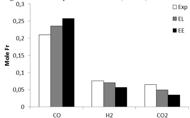
Figure 3. Mole fractions at gasifier outlet (AR=0.35, SR=0.0).
