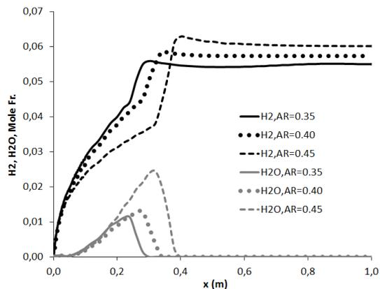
Figure 7. Predicted axial variations of H<sub>2</sub> and H<sub>2</sub>O mole fractions (SR=0.0).
