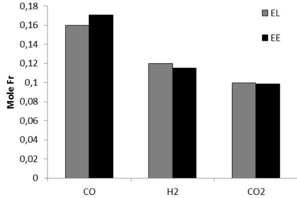
Figure 8. Predicted mole fractions at gasifier outlet (AR=0.40, SR=0.1).
