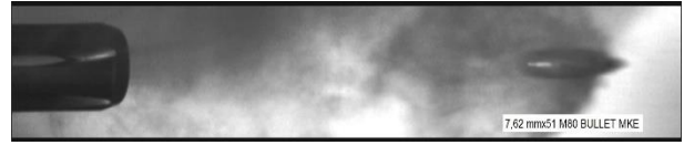
Figure 7. The motion of a 7,62 mm M80 bullet during intermediate ballistic phase (courtesy of Mr. Osman Başak).
