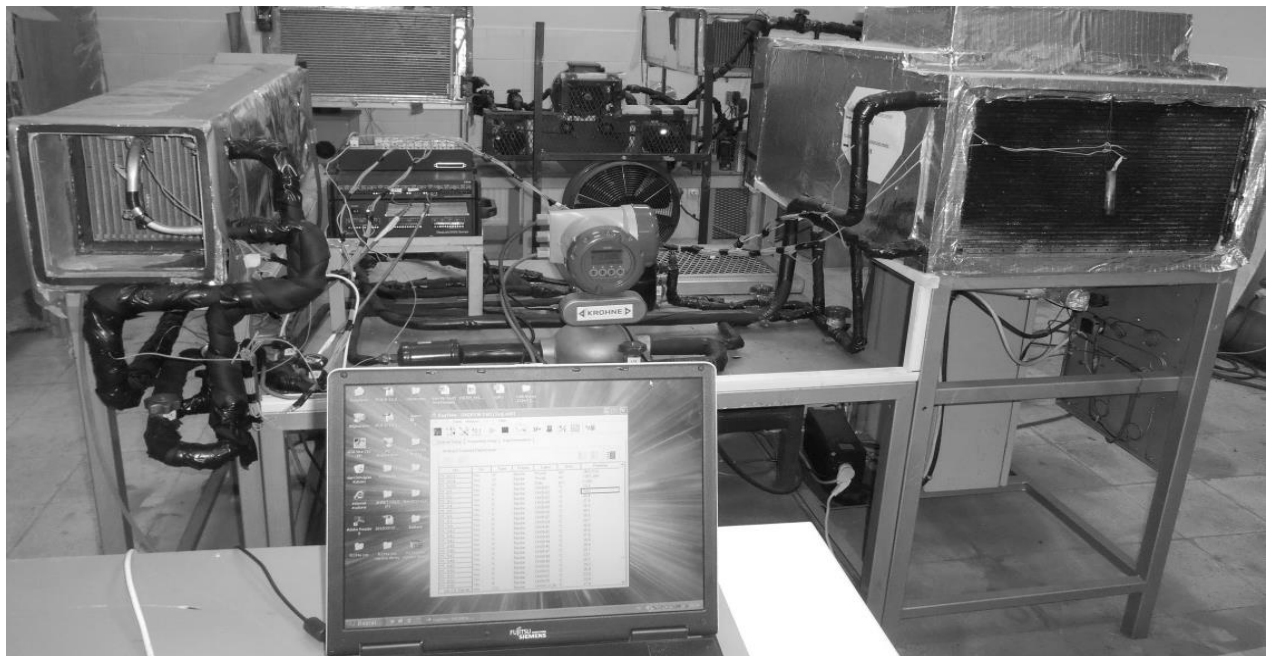
Figure 1. Photograph of the experimental AAC system.
