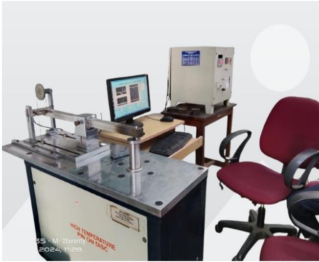
Figure 3. Pin on Disc setup
