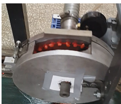
Figure 2. A view from the experiments conducted with universal vacuum disk equipped with adaptors at 4 mm for corn seeding
