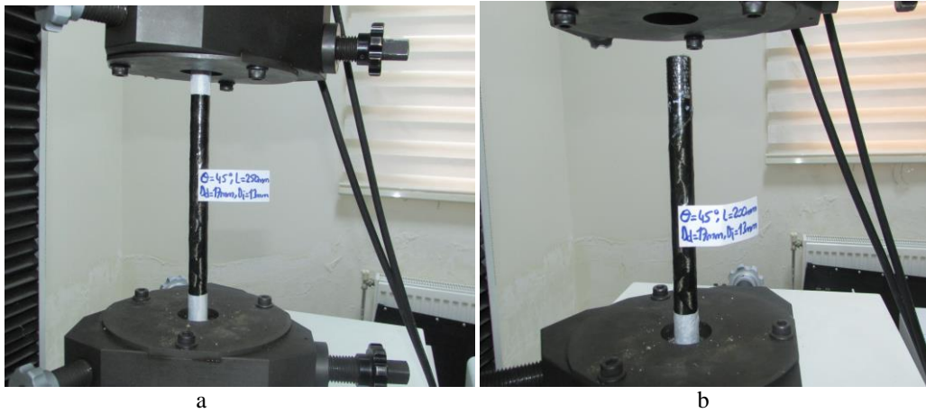
Figure 3. The samples of 250 mm long carbon / epoxy; a) before torsion, b) after torsion
