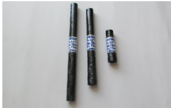
Figure 2. A test specimens of carbon/epoxy
