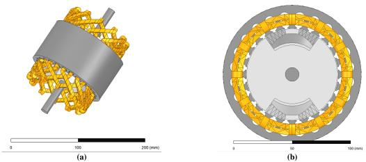
Figure 7. The full modeling 3D image for the CPSG, (a) 3D image, (b) front view of generator.
