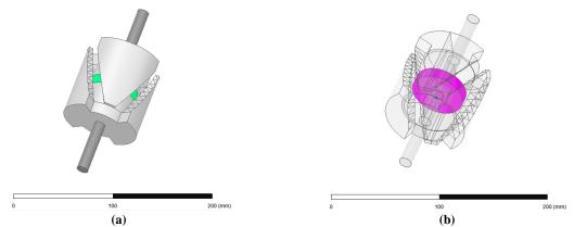
Figure 6. The rotor (a), and pole structure (b) of CPSG.
