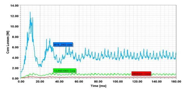
**Figure 9.** The core loss behavior of CPSG designed with M19\_24G, Amorphous and JFE super core materials.
