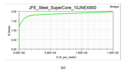
**Figure 2.** B–H curve comparison of the core materials, (a) M19\_24G, (b) 2605SA1 core, (c) 10JNEX900 core.
