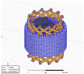
Figure 8. Mesh refinement of CPSG.
