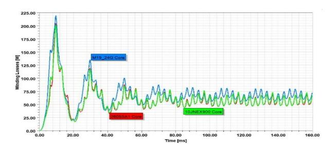
**Figure 10.** The copper loss behavior of CPSG designed with M19\_24G, Amorphous and JFE super core materials.
