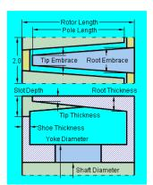
Figure 5. Sizing parameters of claw pole rotor [40].
