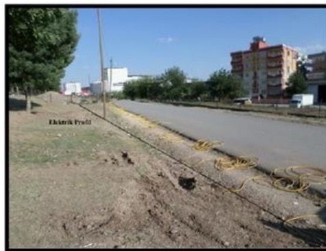
Figure 13. Measurement in the field with the multi-electrode electrical resistivity method
