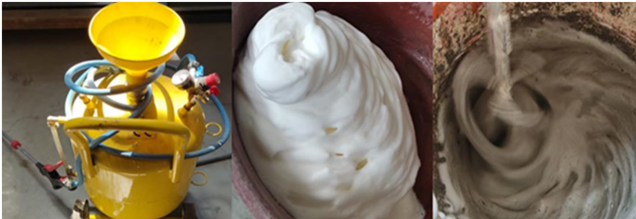
Figure 4. Foam and foam concrete mixture
