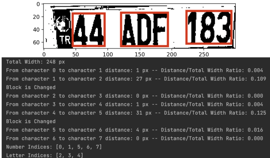
Fig. 9. The process of identifying plate blocks.
