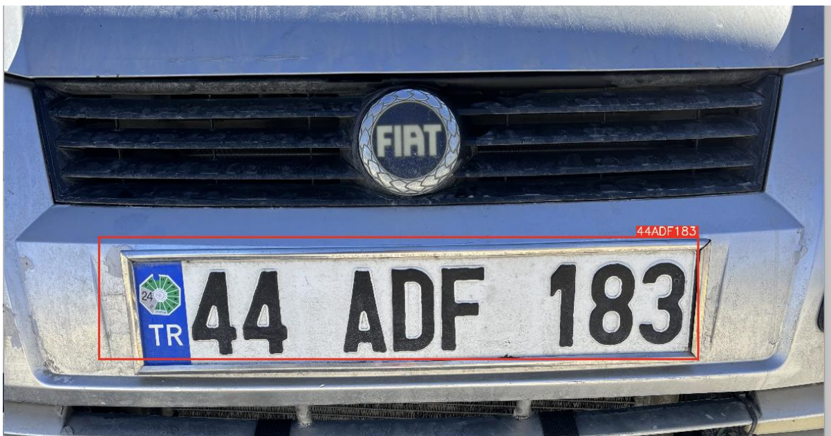
Fig. 23. Image of a vehicle with completed license plate recognition.
