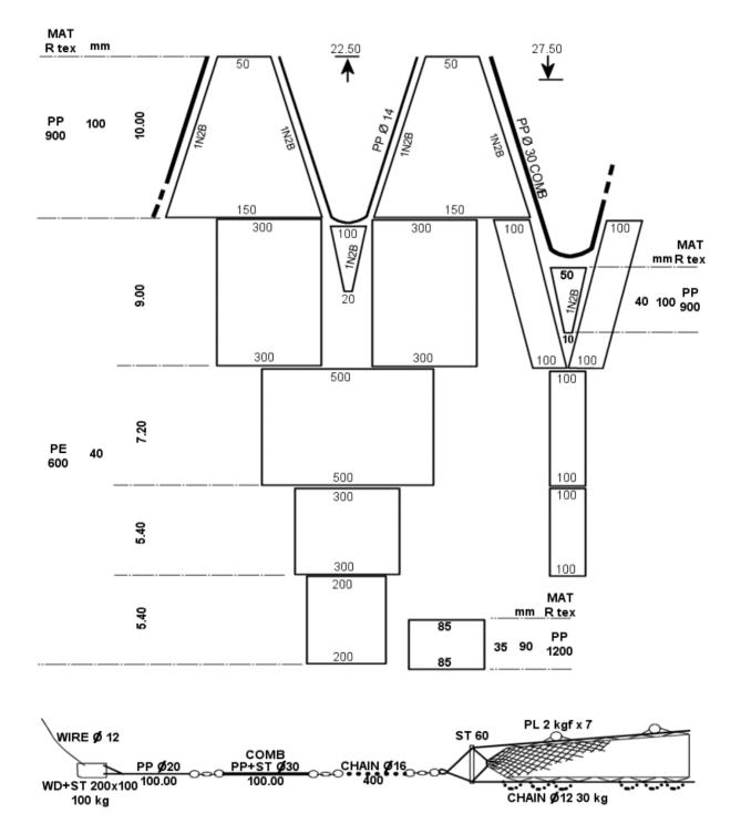
Figure 2. Technical plan of commercial demersal trawl used in the Black Sea coasts
