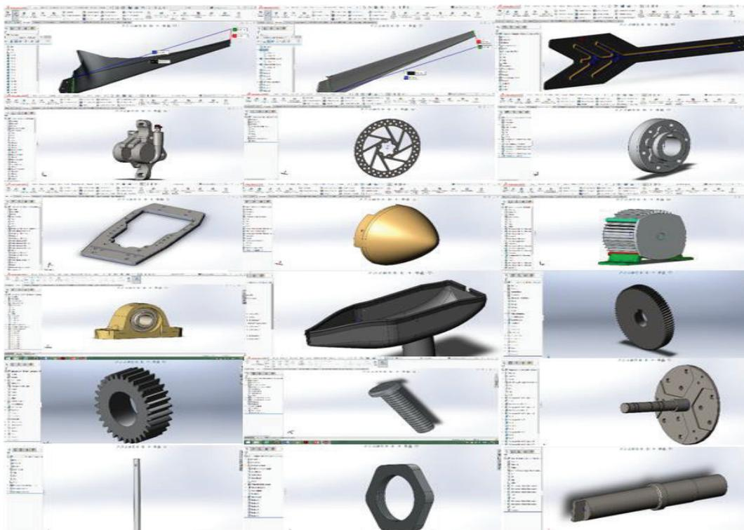
Figure 1. Solid models of wind turbine components
