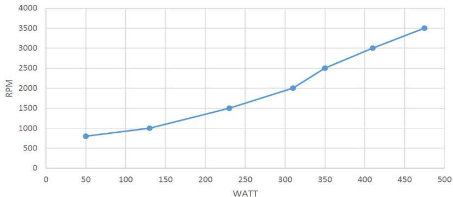
Figure 18. Alternator power output according to the rotation speed
