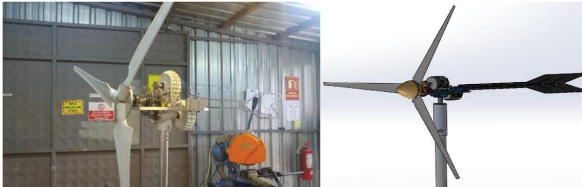
**Figure 22.** Designed and manufactured rotor turbine
