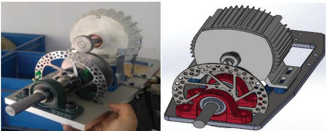
**Figure 20.** Designed and manufactured plate support element
