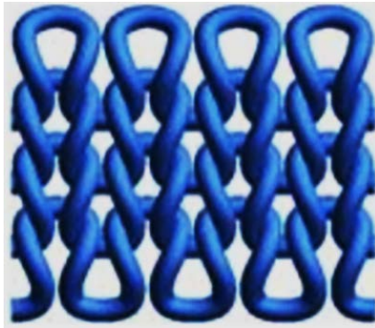
Figure 12. 3D simulation of weft knitted fabric based on NURBs curve [25]
