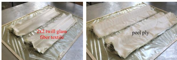
Figure 5. a) Use of release film and tape in composite production b) Arrangement of U-profile molds
