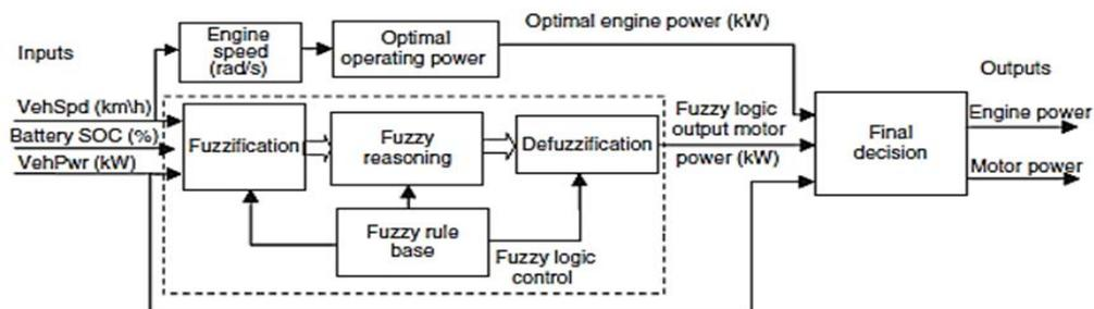
Figure 5. Fuzzy-based control system diagram [11]
