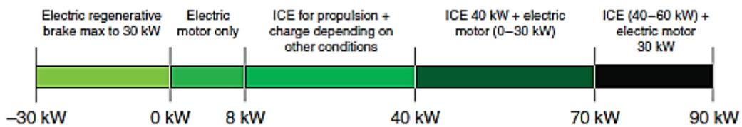
Figure 2. Working principle of hybrid electric vehicle [11]
