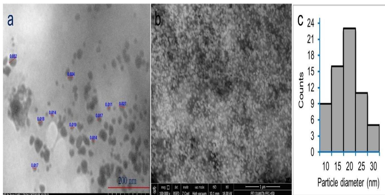
**Figure 3.** TEM (a), SEM (b) and particle size distribution (c) of OB-AgNPs.
