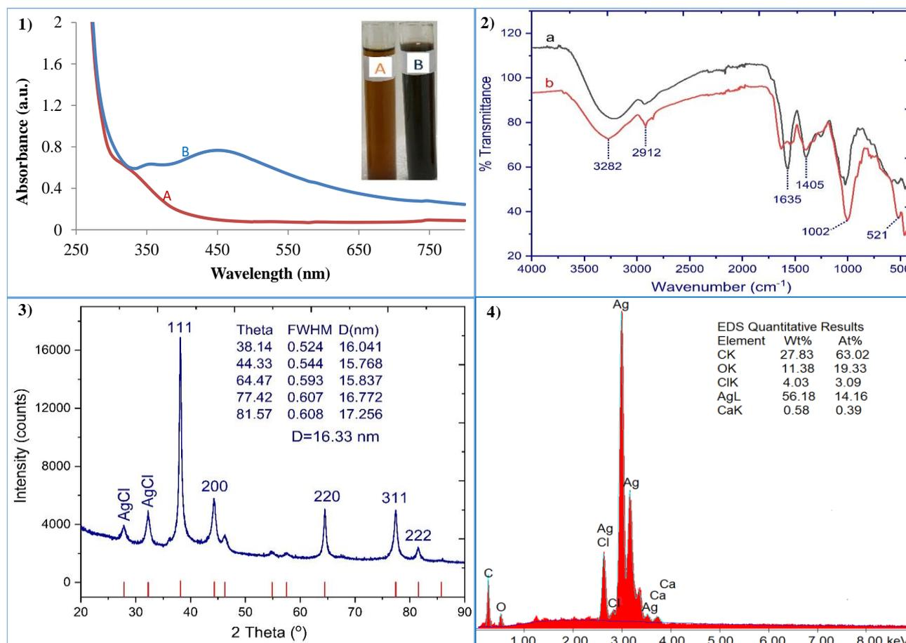
**Figure 1.** UV-Vis spectrum (1), FTIR spectrum of extract (a), nanoparticles (b) (2), XRD pattern (3), and EDX spectrum (4) of OB-AgNPs.
