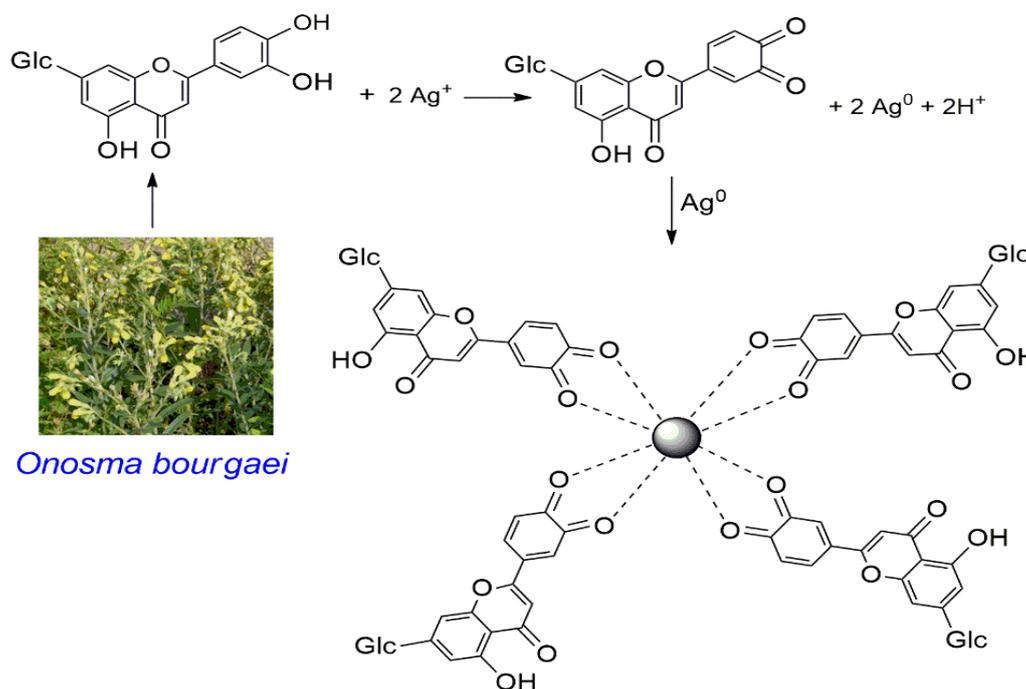
**Figure 2.** Possible reaction mechanism of synthesis of OB-AgNPs.
