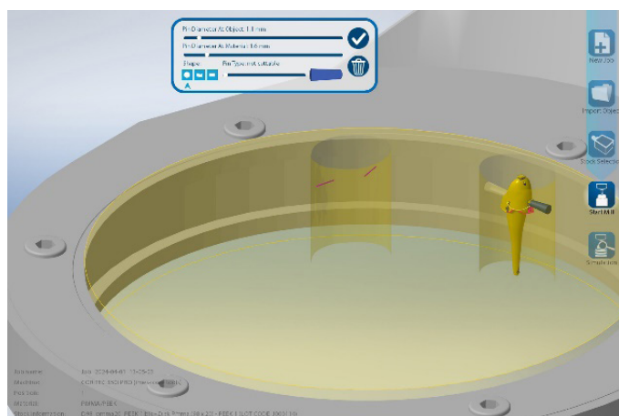
Figure 3. Screenshot of virtual nesting process for custom post-and-core designs with dual sprues in CAD/CAM disc via software program.
