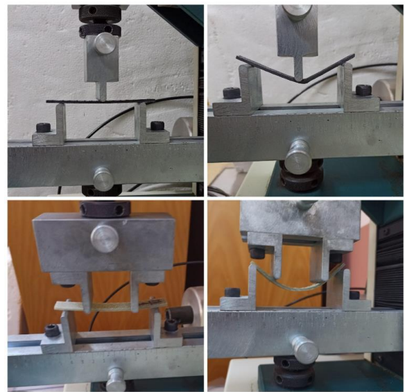
Figure 2. composite samples during 3 and 4-point bending tests
