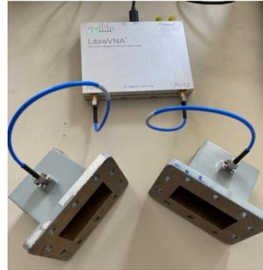
**Figure 3.** Shielding performance measurement mechanism.
