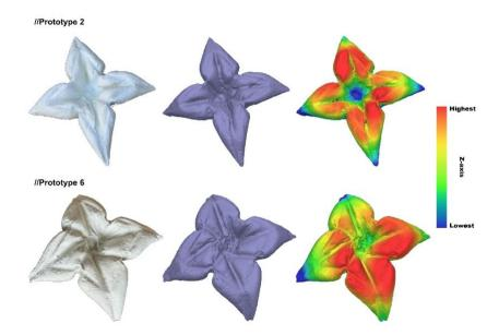
Figure 20: Metashape models using Photogrammetry technique. (Mesh-Textured, Mesh-Solid, Point Cloud-Elevation)
