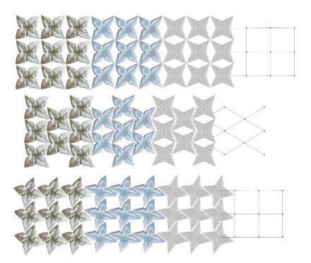
Figure 23: Deployable panel patterns grid, digital pattern, patterns using the physical model. (grid pattern, diamond pattern, grid pattern with angled units).
