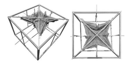
**Figure 14:** Constructed deployable mould system (Photographed by the authors)
