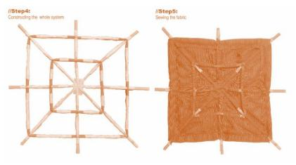
Figure 9: Construction steps of the deployable skeleton structure and sewing. (Photograph by the authors)
