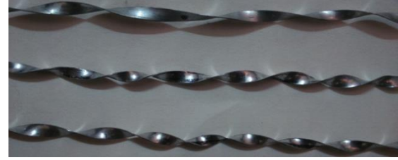
Figure 2. Twisted tapes (twist ratio 3.5, 3, and 2.5).
