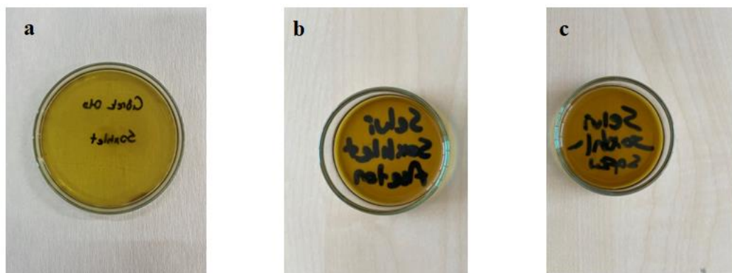
Figure 1. Extract obtained by Soxhlet method with (a) ethanol, (b) acetone and (c) DI water solvent
