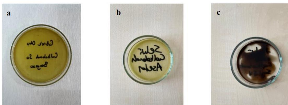
Figure 2. Extract obtained by Maceration method with (a) ethanol, (b) acetone and (c) DI water solvent
