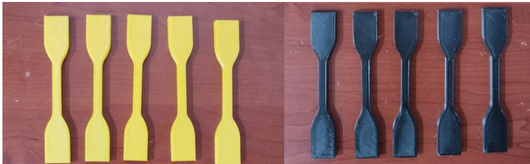
Figure 5 Tensile samples produced by 3D printer (yellow colour ABS filament material, black colour PETG filament material)
