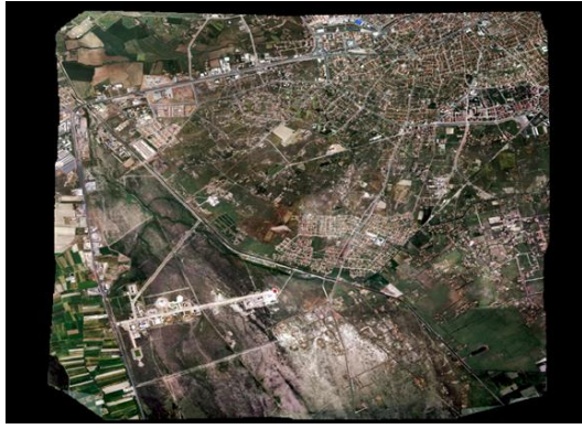
Figure 10. Orthophoto mosaic image produced using digital aerial photographs taken with 25 cm GSD
